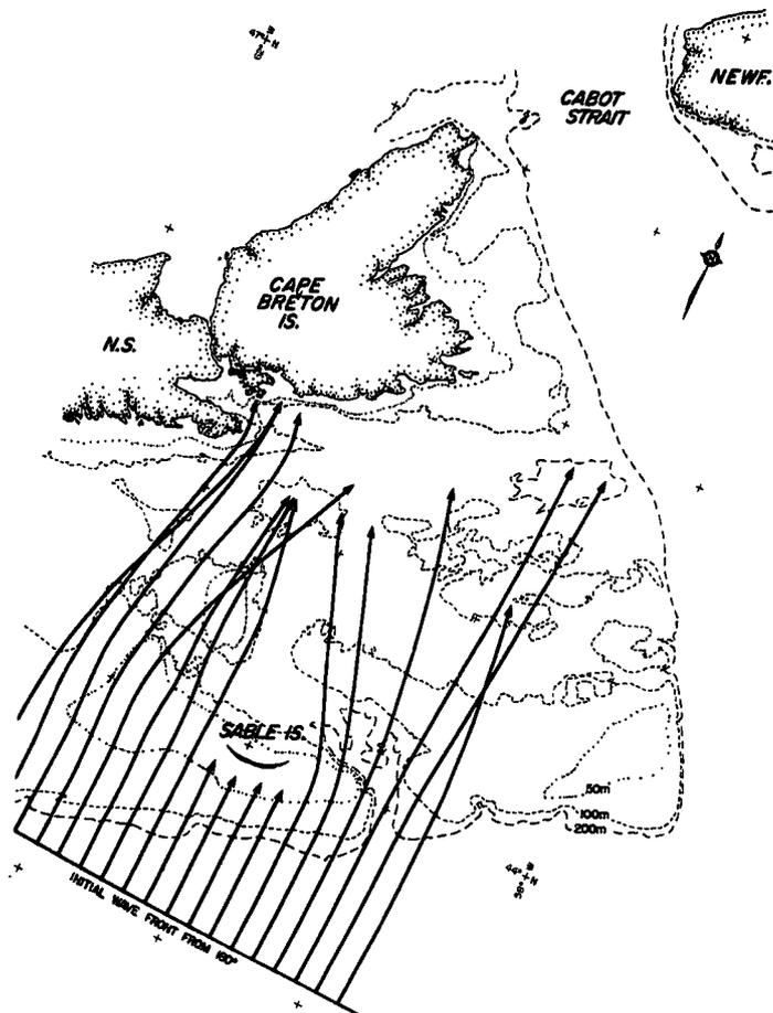
Figure 9. Refraction diagram of a wave front from the south and a wave period of 14 s
